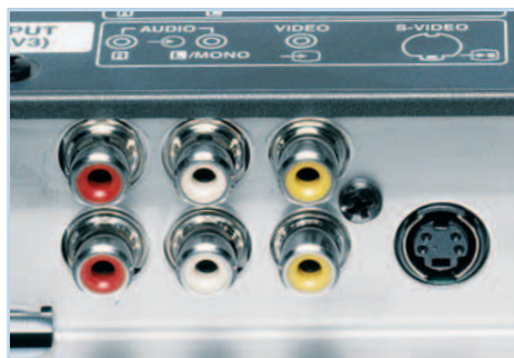
The AV connections are found at the bottom of the panel
